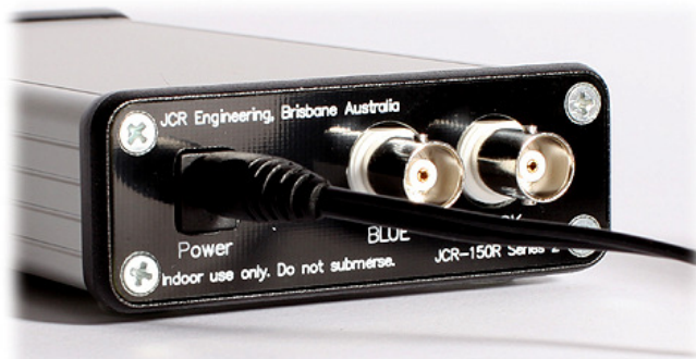
The rear of the 150R unit showing the charger lead. (This must always be unplugged before the unit is used)
